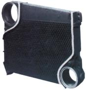
The sections are studded with heat pins that cause the hot gases to swirl about. scrubbing the entire surface for greater heat transfer and maximum operating efficiency.
